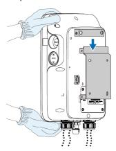
3 Secure the upper and lower mounting plates to the backplate with screws. (Torque:  $1.2 \pm 0.1 \text{ N} \cdot \text{m}$ ).
