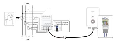
figure 2-4 Connect to a Smart Energy Meter
