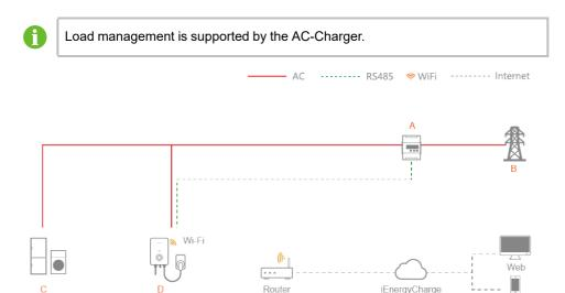
figure 1-5 System topology diagram of Load Balancing
