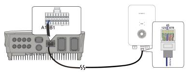
figure 2-5 Connect to an inverter(SHRT)
