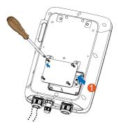
**Step 3** Plug the cable into the port of the power supply which is at the leftmost.
