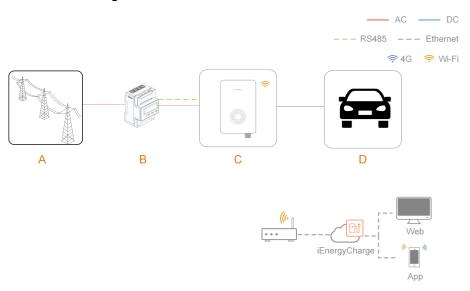
figure 1-3 System topology diagram of EV charger
