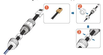
figure 2-3 RJ45 screw connector(B)
