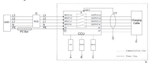
figure 2-1 Circuit diagram
