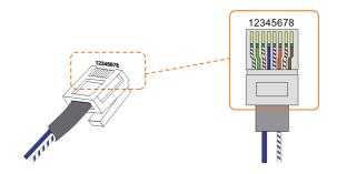
Step 2 Insert the RJ45 connector to the RJ45 jack.
