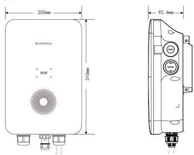
figure 1-2 Dimensions (in mm)
