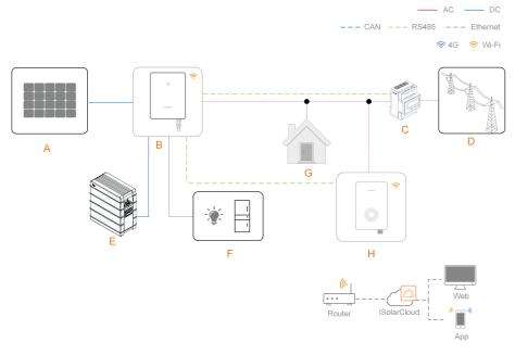
figure 1-4 System topology diagram of the solar-storage-charging solution
