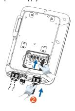
**Step 4** Adjust the cable to a suitable length, and strip off the insulation of the cable to prepare for cable connection terminals.
