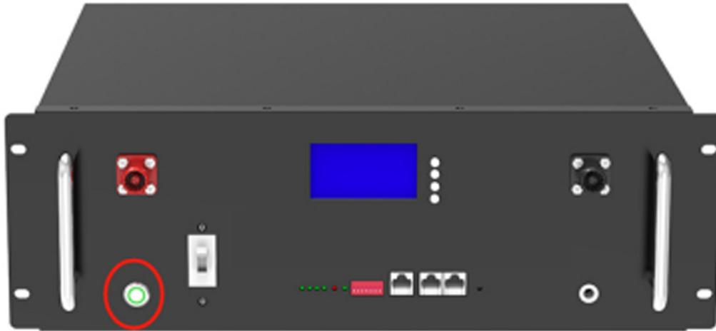
Step 3. Pull DC breaker to “ON” position, then system can begins to work.
