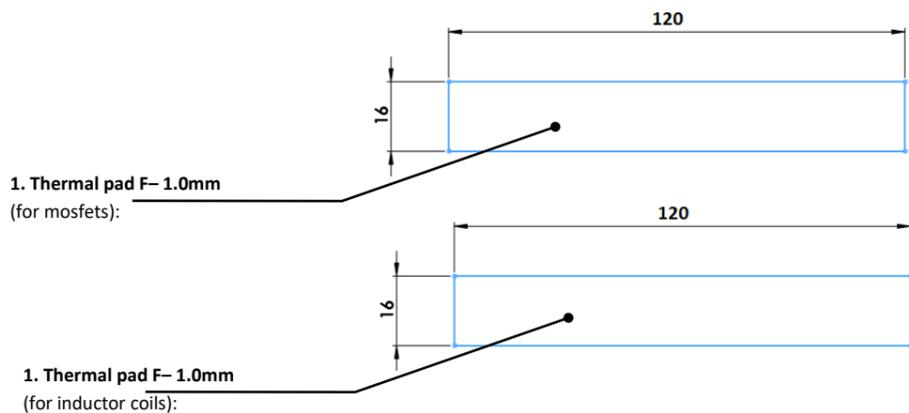
Place 1mm thermal pads in larger strips over marked area and make sure all mosfet chips are covered.
