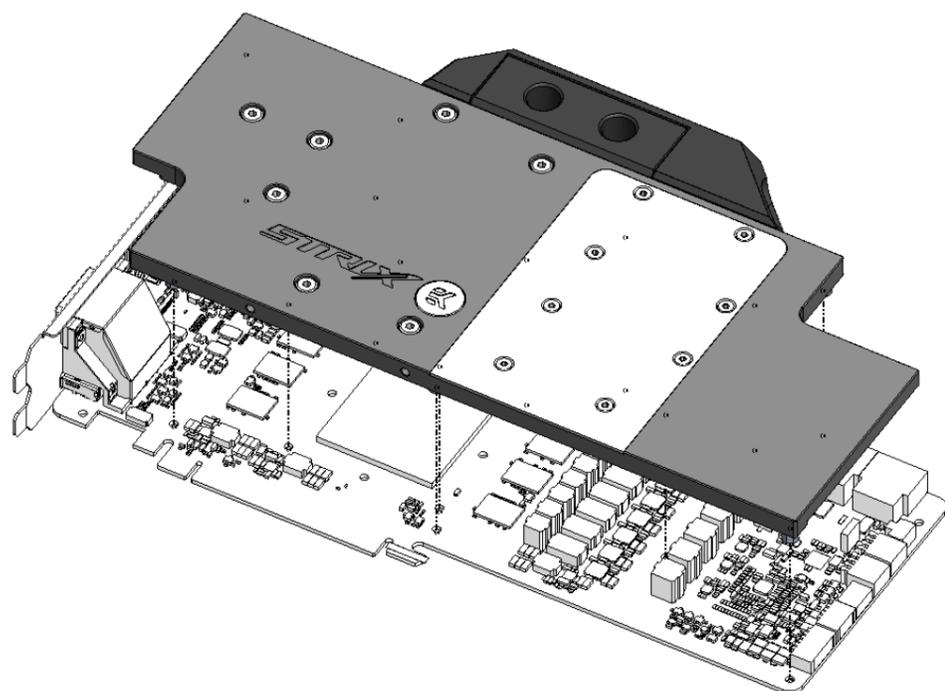
**2. ATTACHING THE BLOCK TO THE GRAPHIC CARD.** Use a Philips screwdriver screw with the enclosed M2,5x4 AX1 screws. EKWB recommends users to start tightening the screws around the GPU core and continue outwards. Always use a plastic washer under each and every screw! If the washer is already present on the circuit board (usually around the four GPU core screw holes) there is no need for additional washer.
