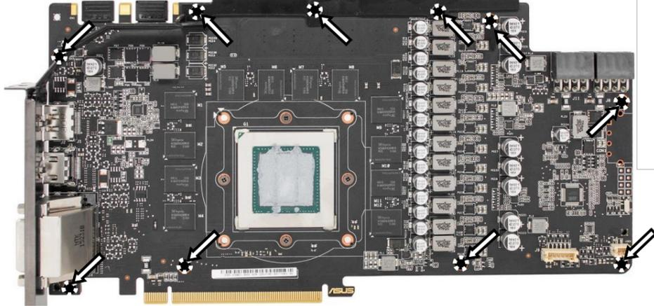
Please do not forget to remove stock-glued washers from the front side of the pcb, if present!!!
