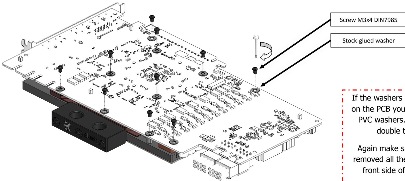
If the washers are not stock-glued on the PCB you must use enclosed PVC washers. Be careful not to double the washers!
