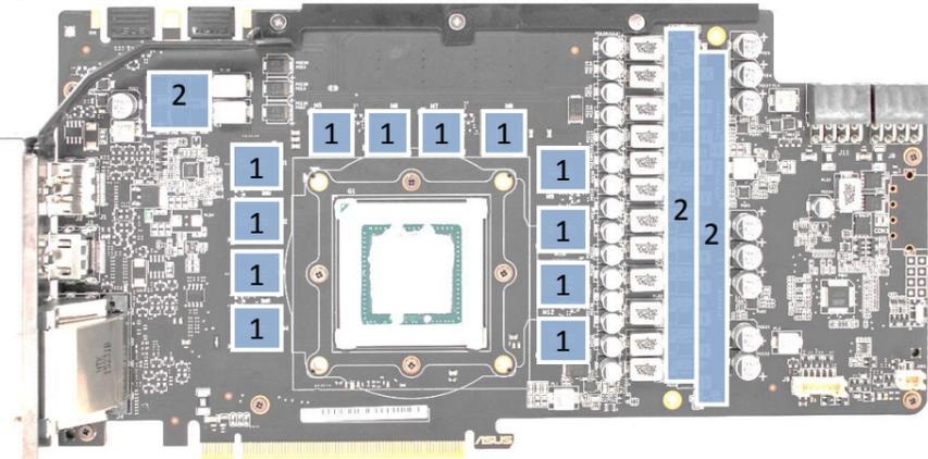
2. PLACING THE BLOCK ON TO THE GRAPHICS CARD. Carefully position the water block with preinstalled 2.5mm standoffs on to the graphics card. During this process please make sure you align mounting holes on the PCB with holes on the water block (same applies for other tops). Also pay attention not to use too much force by pressing the block down to the PCB. Chip dies are prone to cracking.
