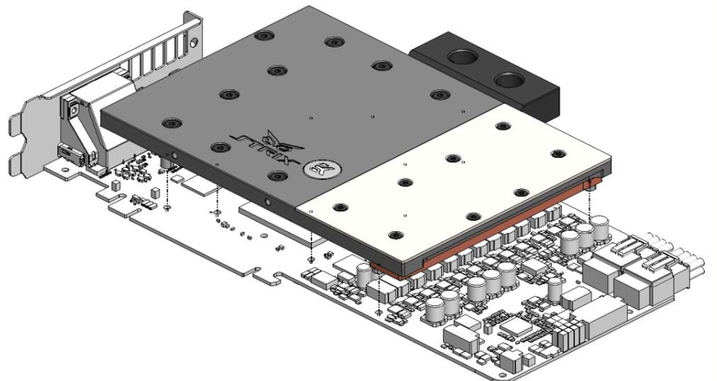
3. ATTACHING THE BLOCK TO THE GRAPHIC CARD. Use a Philips screwdriver with the enclosed M3x4 DIN 7985 screws. EKWB recommends users to start tightening the screws around the GPU core and continue outwards. At short top version (plexi) the encircled screws are to be left out.
