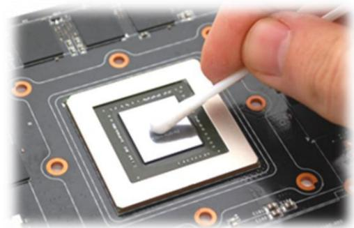
3. APPLYING THERMAL COMPOUND. Wipe off the remains (by using non-abrasive cloth or *q-tip*) of the original thermal compound until the components and circuit board are completely clean. Apply thermal compound: lightly coat **NVIDIA** GPU chip with enclosed EK-TIM Ectotherm thermal grease. EKWB recommends to apply thermal grease in cross form for best performance (see sample picture).
