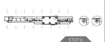
Place the active backplate on the PCB and make sure all holes are aligned. Position an M2.5  $\times$  8 AX1 screw into each of the five (5) mounting holes (as shown in the image) and tighten them evenly with a Phillips head screwdriver.
