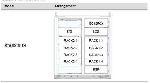
Note: RACK x-x represents a 1P64S PACK. S/G stands for switch gear, SC125CX for DC/AC power converter unit, LCS for liquid cooling unit, and BSP for power distribution box.
