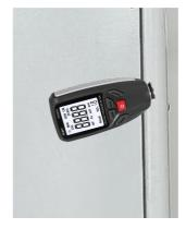
**d.** When applying multiple layers of paint, wait for each layer to dry completely before applying the next. The total thickness of the primer and finish paint must be at least 240μm.
