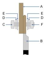
Figure 5-4 Copper-to-aluminum adapter terminal connection
