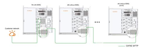
Figure 5-9 Networking Diagram Between ESSs
