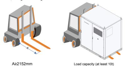
Figure 4-4 Handle with Forklift (Side)
