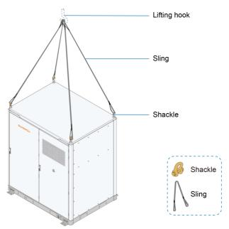
Figure 4-6 ESS Hoisting
