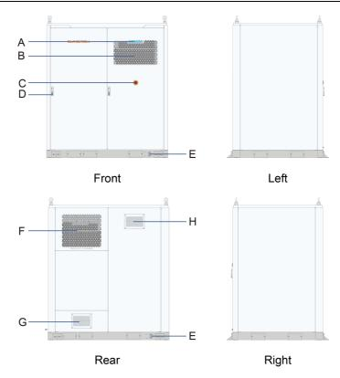
Figure 2-2 ESS External Design
