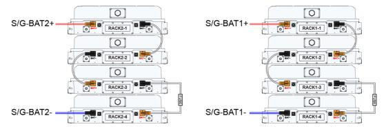
Figure 6-5 PACK Wiring Diagram
