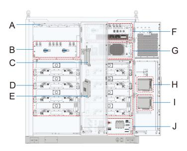
Figure 2-6 Internal Structure of the ESS
