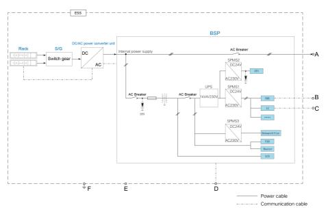
Figure 5-1 Wiring Diagram
