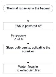
Figure 8-5 Control Logic of the Backup Protection System
