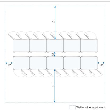
Figure 4-3 Space Required for ESSs in Two Rows
