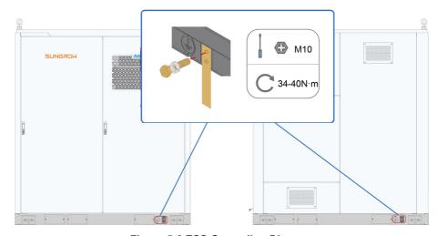
Figure 5-6 ESS Grounding Diagram
