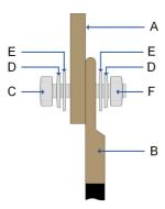
Figure 5-3 Copper cable terminal connection sequence
