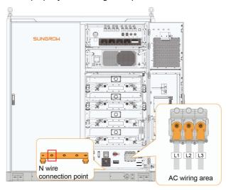
Figure 5-7 AC Wiring Area
