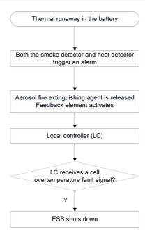
Figure 8-4 Control Logic of the Fire Extinguishing System
