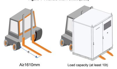
Figure 4-5 Handle with Forklift (Front)
