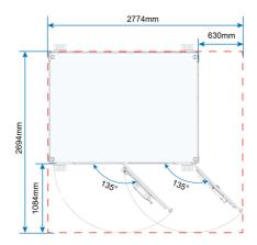
Figure 2-4 Dimensions of ESS with its Door Fully Open
