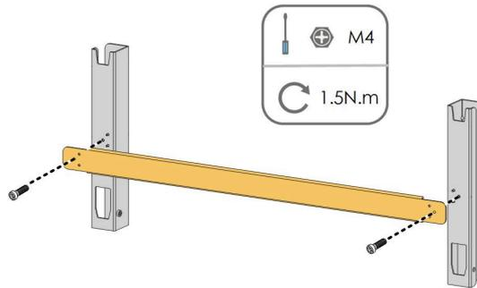
**step 2** Level the assembled mounting-bracket by using the level, and mark the positions for drilling holes on the PV bracket. Drill the holes by using a hammer drill.
