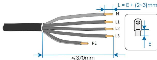
**step 6** Make the cable and crimp OT/DT terminal.
