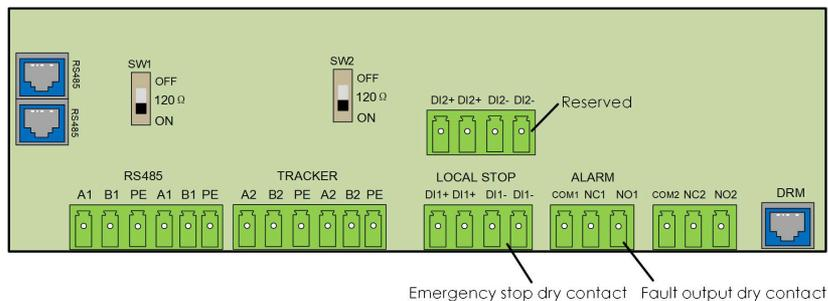
**DO terminal (fault output dry contact):** The relay can be set to output fault alarms, and user can configure it to be a normally open contact (COM & NO) or a normally closed contact (COM & NC). If the earth fault occurs, the DO dry-contact will switch on automatically to signal the external alarm. The LED will turn red and a beeping sound will alarm until the fault is rectified, for internet connected products the error will also be sent to the portal.
