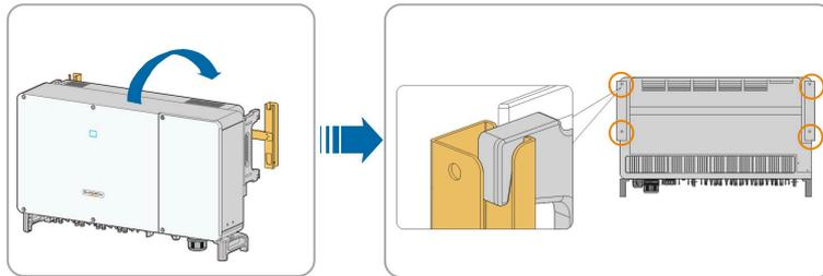
**step 4** Fix the inverter with screws.
