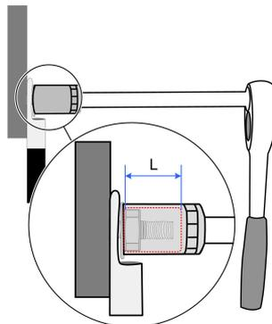
**step 8** Gently pull the cable backwards to ensure firm connection, and fasten the swivel nut clockwise.
