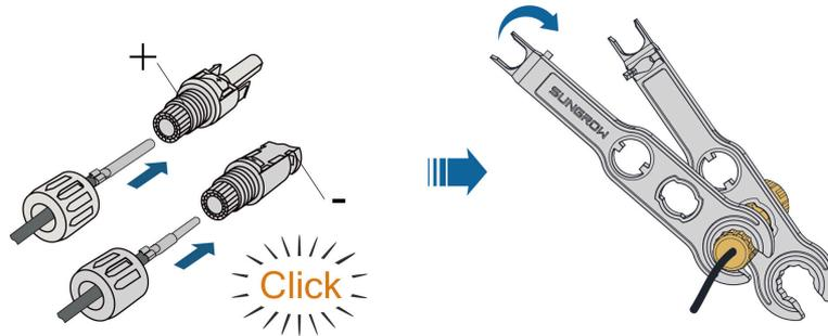
**step 4** Check for polarity correctness.
