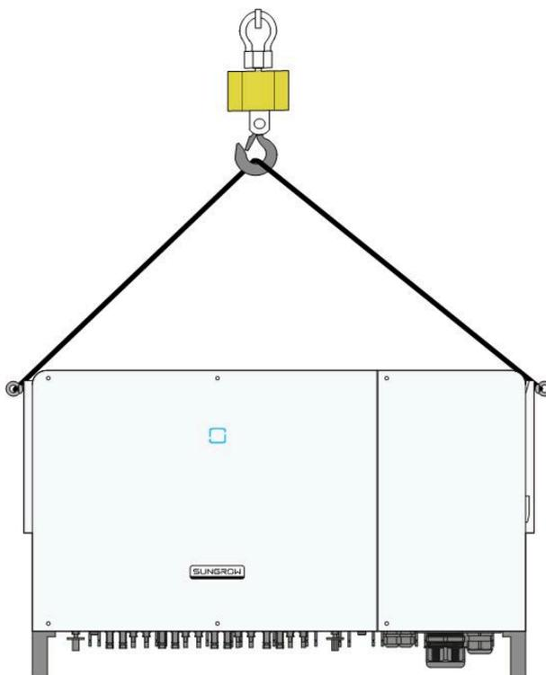
**step 4** Remove the lifting rings and reassemble the sealing screws released in Step 1.
