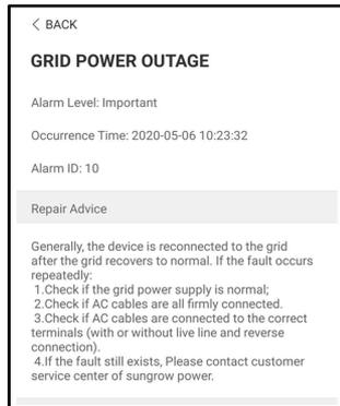
**figure 7-9** Detailed Fault Alarm Information
