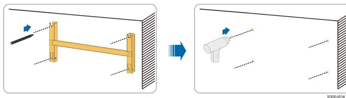
**step 3** Insert the expansion bolts into the holes and secure them with a rubber hammer. Fasten the nut with a wrench to expand the bolt. Remove the nut, spring washer, and flat washer, and store them properly.
