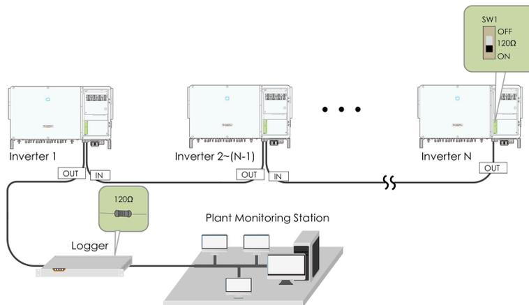
**figure 5-7** Configuration of Dip Switch ( $N \geq 15$ )
