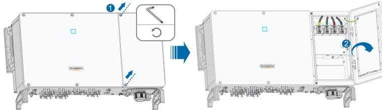
**step 3** Keep the wiring compartment open during wiring through the limit lever attached to the cover.
