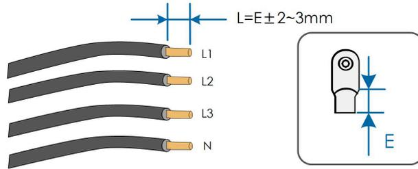
**step 6** Make the cable and crimp OT/DT terminal.
