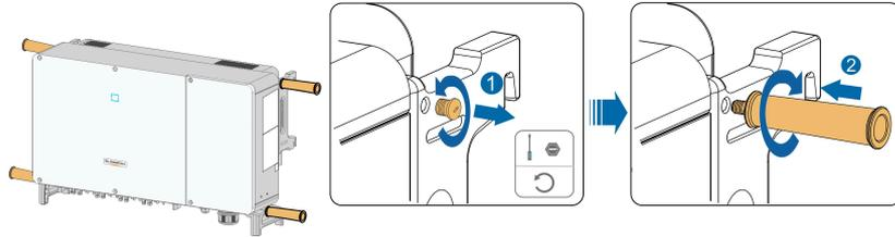
**step 2** Lift and move the inverter to the destination by using the side and bottom handles as well as the four installed handles.
