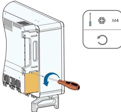
**step 3** Press the tab of the latch hook, unplug the cable connection joint outwards, and loosen the screw on the fan holder.
