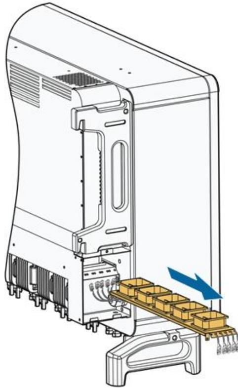
**step 5** Reinstall the fan back to the inverter in reverse order and restart the inverter.
