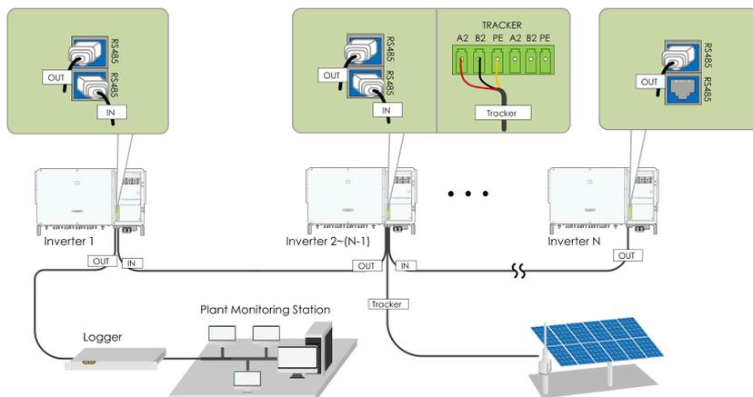
**figure 5-6 Multi-inverter Communication System 【RS485\_1 Interface ( RJ45 ) 】【**
