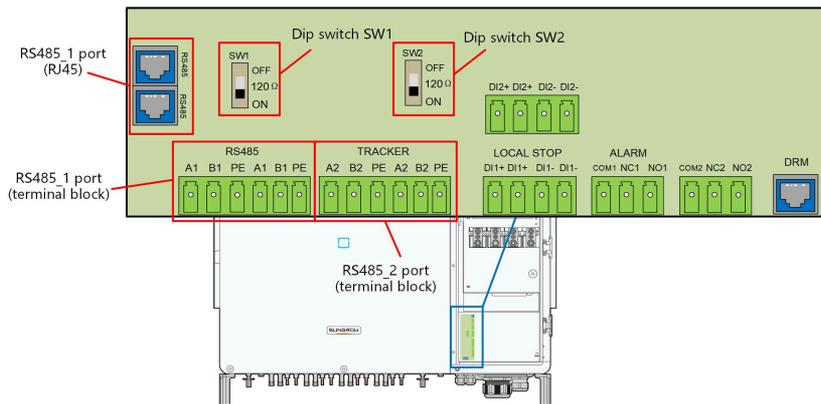
The inverter is equipped with two groups of RS485 communication port for external communication connection, which are RS485\_1 port and RS485\_2 port.
