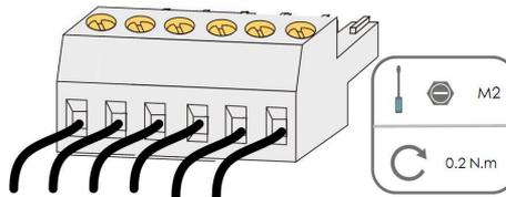
**step 4** Insert the terminal base into the corresponding terminal.
