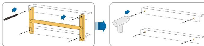
**step 3** Secure the mounting-bracket with bolts.
