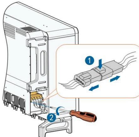
**step 4** Pull out the fan module, clean the fans with soft brush or vacuum cleaner, and replace them when necessary.
