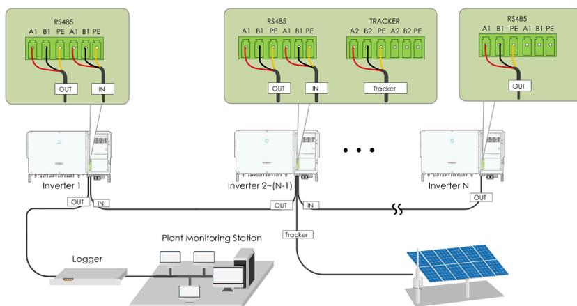
**figure 5-5 Multi-inverter Communication System 【RS485\_1 Interface ( Terminal Block ) 】【**
