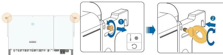
**step 2** Lead the sling through the two lifting rings and fasten the tie-down strap.
