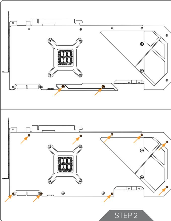
Remove the nine screws with Phillips and Torx head screwdrivers and carefully detach the stock backplate from the PCB.
