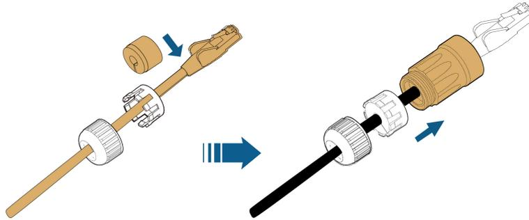
**Step 5** Insert the RJ45 plug into the front plug connector until there is an audible click and tighten the housing. Install the gasket and fasten the swivel nut.
