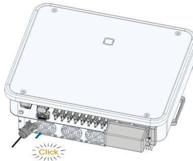
**Step 3** Pull cables outwards to confirm whether they are fastened firmly.
