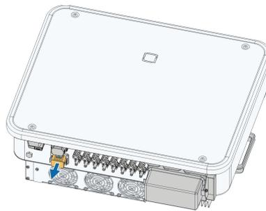
**Step 2** Insert the COM connector into **COM** terminal on the bottom of the inverter until there is an audible click.
