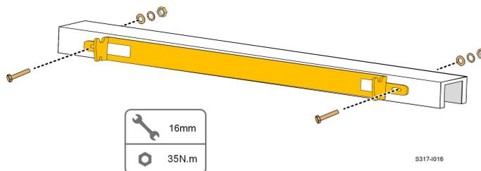
**Step 4** Secure the steel u-channels to the pole with bolts and clamps.
