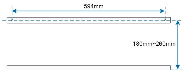
**Step 2** Secure the mounting-bracket to the steel u-channel with bolts.
