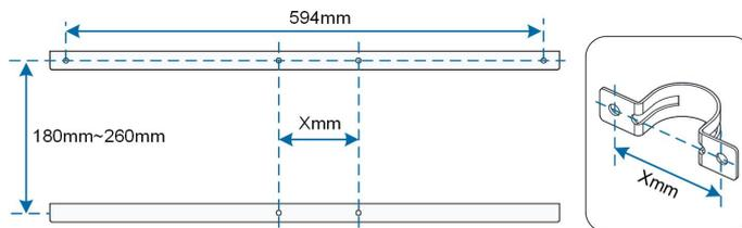
**Step 3** Secure the mounting-bracket to the steel u-channels with bolts.
