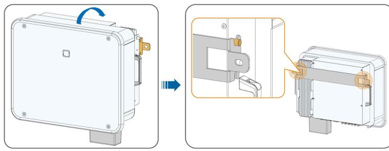
**Step 3** Fix the inverter with screws.
