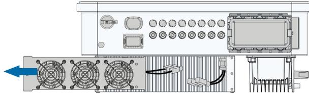
**Step 5** Reinstall the fan back to the inverter in reverse order and restart the inverter.
