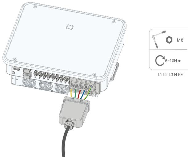
Ensure that the depth L of the socket used is not less than 18mm.
