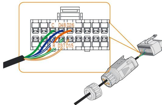
**Step 6** Pull the wires outward to check whether they are firmly installed.
