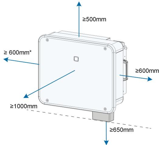
\*When this distance is less than the distance shown, lift the inverter off the stand or wall before maintaining fans.
