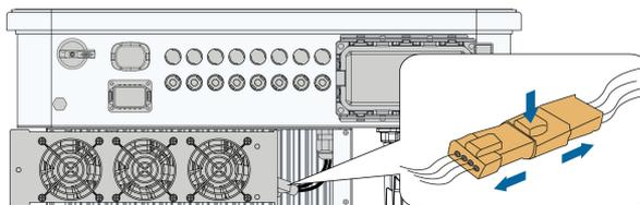
**Step 4** Pull out the fan module, clean the fans with soft brush or vacuum cleaner, and replace them when necessary.
