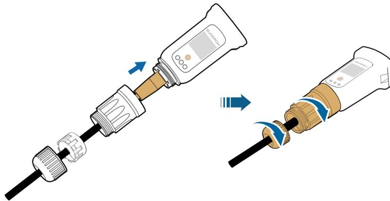
**Step 6** Remove the waterproof lid from the **COM1** terminal and install WiNet-S.
