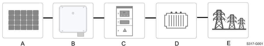
figure 2-1 Inverter Application in PV Power System
