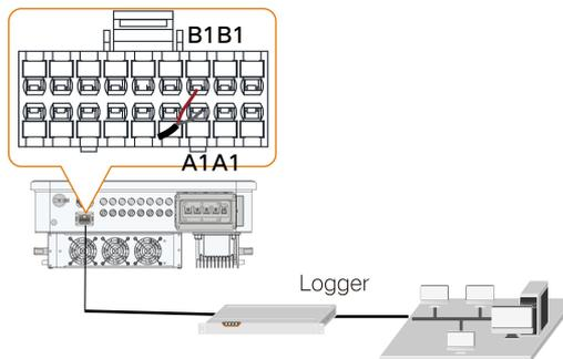
In case of multiple inverters, all the inverters can be connected via RS485 cables in the daisy chain manner, as shown in the following figure.
