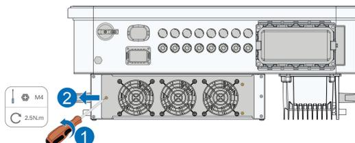
**Step 3** Press the tab of the latch hook, unplug the cable connection joint outwards, and loosen the screw on the fan holder.
