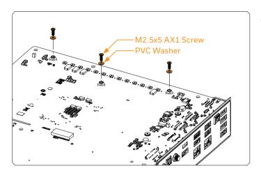
**Mosfet part:** Use three (3) M2.5 X 5 AX1 Screws and PVC washers. Tighten the screws evenly.
