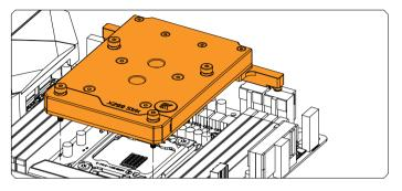
Place the EK-Quantum Momentum ROG Strix X299-E Gaming II series water block to the motherboard or vice versa (as shown on the photo). Make sure that mounting holes are aligned.
