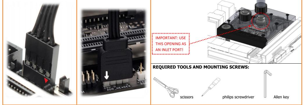
For the EK-FB ASUS Z270I Strix Monoblock series water block to operate properly the G1/4 port nearest to the right edge of the water block **MUST BE USED AS THE INLET** PORT. EK recommends the use of EK-ACF fittings. When using fittings other than EK-ACF series please use hose clamps or appropriate substitute to secure the tubing to the barb. The use of biocide containing and corrosion inhibiting coolant is always recommended for any liquid cooling system.
