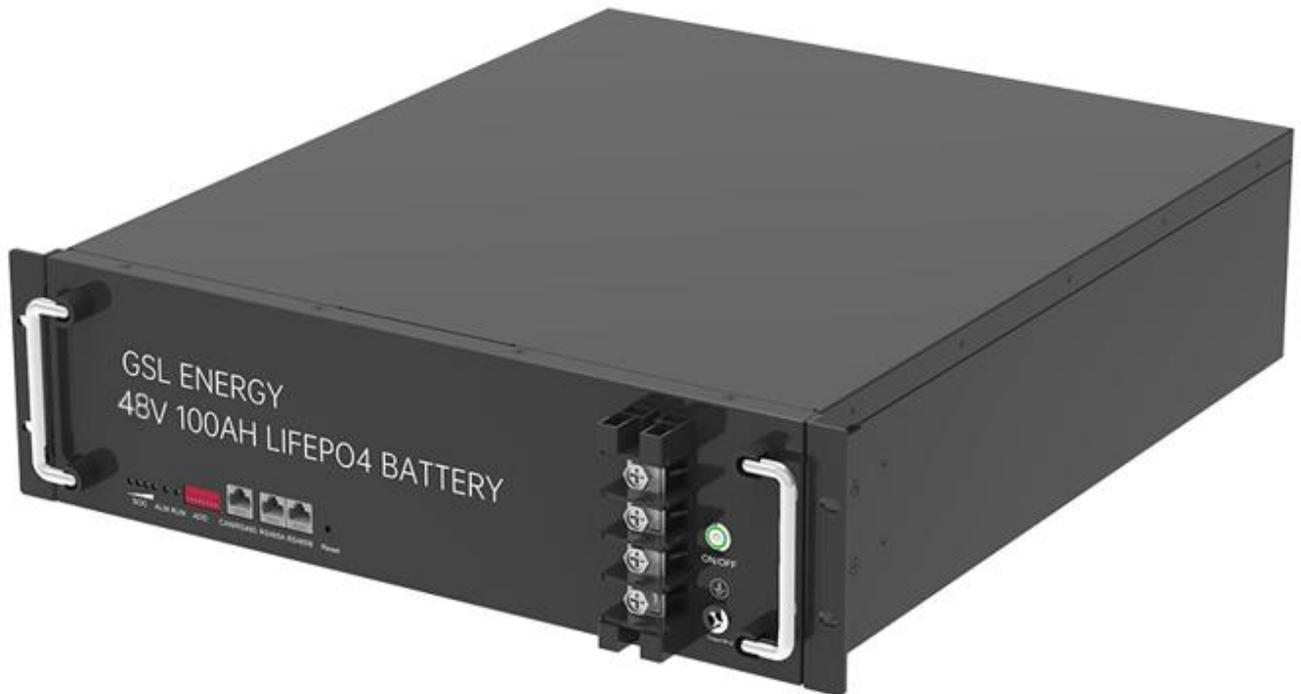
The **ZN-P48100ESA1** 48V 100Ah ( 4.8kwh ) lithium ion phosphate battery energy storage system can be combined in 16pcs ( to max 76.8kwh ) parallel to provide green power supply for solar home storage system via connecting with different 48Vdc solar hybrid on-off storage inverters.
