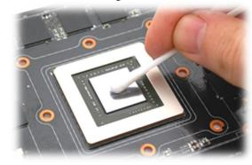
3. APPLYING THERMAL COMPOUND. Wipe off the remains (by using non–abrasive cloth or *q-tip*) of the original thermal compound until the components and circuit board are completely clean. Apply thermal
