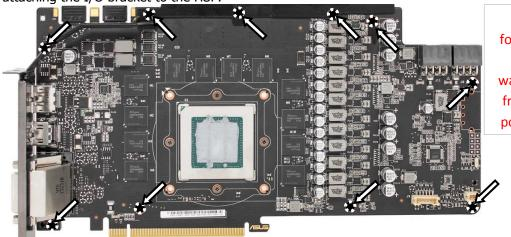
Please do not forget to remove stock-glued washers from the front side of the pcb, if present!!! 2. CLEANING THE PCB. Carefully detach the original stock cooler after removing **all** screws securing it to the board. Wipe off the remains (by using non–abrasive cloth or *q-tip*, as shown on sample photo) of the original thermal compound until the components and circuit board are completely clean. EKWB recommends the use of denatured alcohol for removing TIM leftovers.
